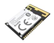
MS88SF2 is advanced, compact (23.2mm  $\times$  17.4mm  $\times$  2mm), highly flexible, ultra-low power wireless BLE 5.0 Module based on nRF52840 SoCs. Its powerful 32-bit ARM Cortex<sup>TM</sup> M4F CPU, a 1 MB flash memory, a 256KB RAM and integrating a 2.4 GH transceiver offers the perfect solution for Bluetooth connectivity.
